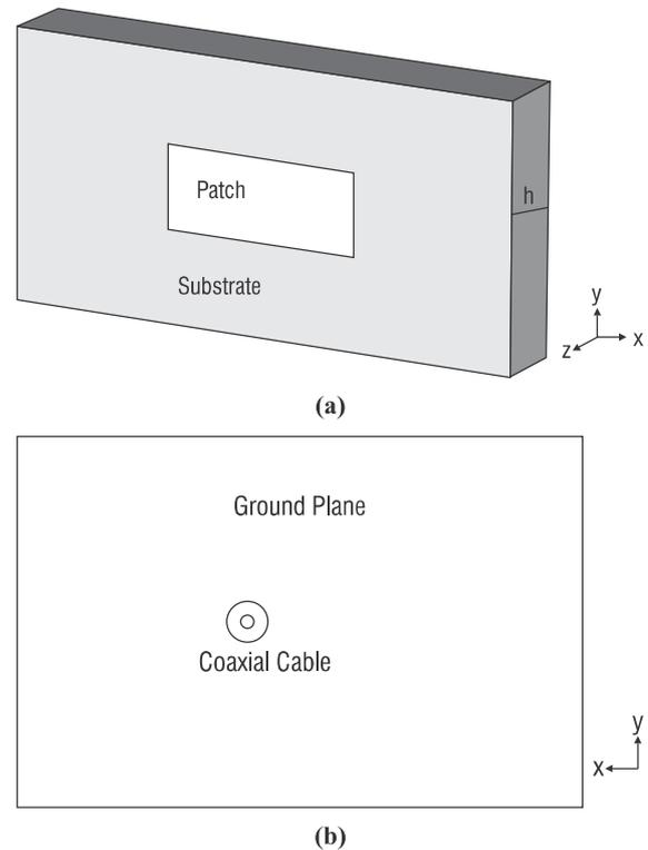
**Fig 1: The Simple rectangular antenna (a) Perspective View (b) Back View**
