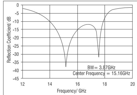
**Fig 4: Return Loss of the proposed antenna**
