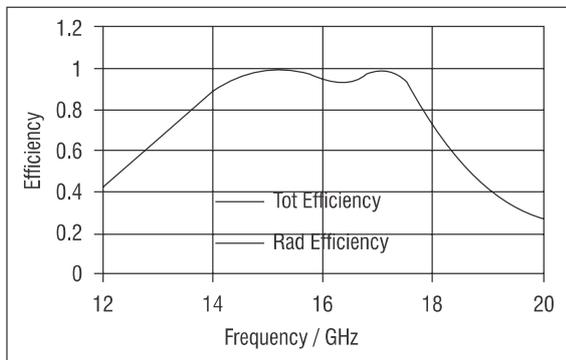
**Fig 6: Efficiency of the proposed antenna**
