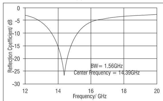
**Fig 2: Return loss of Reference patch antenna**
