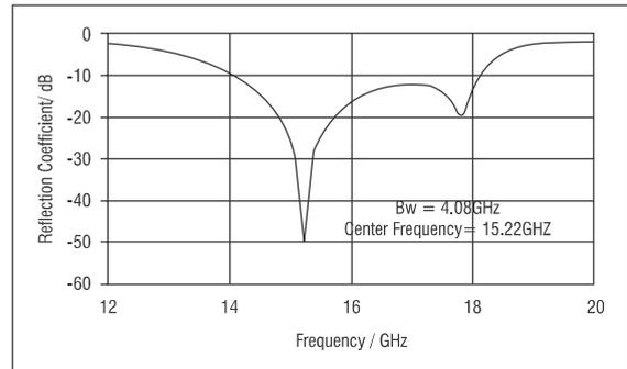
**Fig 8: Return loss of optimized antenna**
